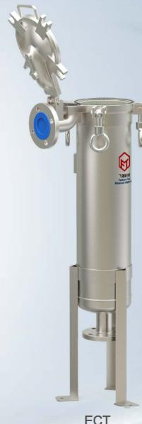
*ECT / ECTG single-bag filter housings with top inlet and bottom outlet are the best choice for cost-effective industrial and commercial applications. Cast construction creates a compact, yet heavy-duty design. The cover directly compresses the filter bag seal-ring, eliminating the possibility of bypass. ECTG housings provide lower pressure loss, making it suitable for sanitary, high viscosity and low pollutant content applications.*
