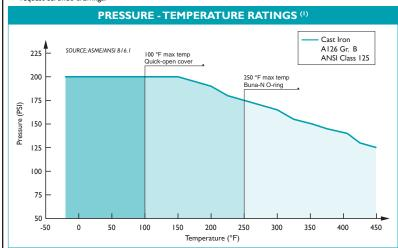
This chart displays the pressure-temperature ratings for the strainer's body material per ANSI B16.1. Max
