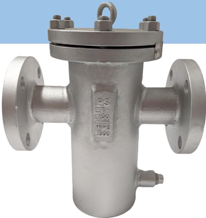
The XSC-BSW Series Simplex Basket Strainer is very basic and cost-effective unit. Designed to ANSI B16.34 with flanges to ANSI B16.5 and tested in accordance with API 598.
