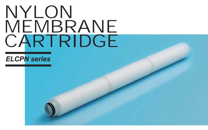
Feature-Tec's ELCPN hydrophilic pleated Nylon 6.6 membrane filter cartridges do not contain any surfactants or wetting agents. This reduces the cleaning time and the cost of the membrane cartridge. ELPCN Nylon membrane filter cartridges are ideal as pre- and final filter for the filtration of Ultrapure water, chemicals and in medical applications.
