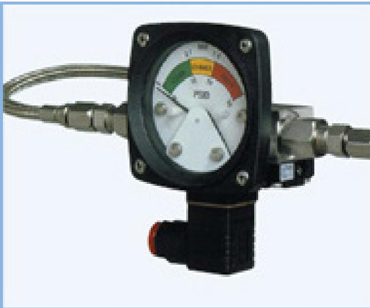
Hayward Flow Control differential pressure gauge and switch assemblies are for use on simplex and duplex bag and cartridge filter housings where differential pressure readings are desired for visual confirmation as well as providing electrical feedback to a control device.
