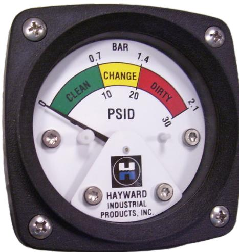
Hayward Flow Control differential pressure gauge assemblies are for use on simplex and duplex bag and cartridge filter housings where differential pressure readings are desired. The differential pressure gauge indicates the difference between influent and effluent pressure conditions, resulting in differential pressure readings used to schedule filter media change-out. The  $\Delta P$  range is 0 - 30 PSID. No adjustments are required.
